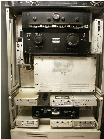
Figure 3 – Basic mechanical configuration showing swing out modules
